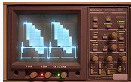
Colour signals mixed with video signal
