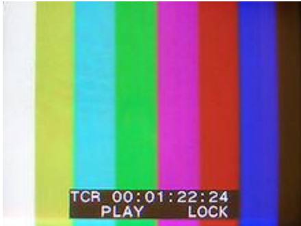
Colour bar generator test signal
